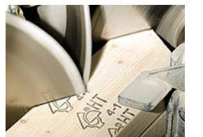
Accurate machine cut rafters make a tight joint for maximum strength and precise construction.
